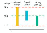
CVR: Reducing the voltage every hour DVR: Reducing the voltage only during select hours
